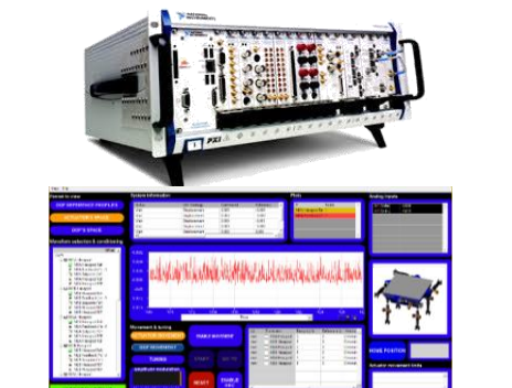
Inner Loop Controller: VZERO MADC hardware and software
