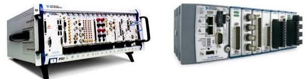
Embedded PXI Chassis and FPGA Controller
